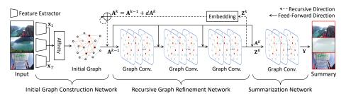
**Fig. 3.** Network configuration of SumGraph, consisting of a initial graph construction network, recursive graph refinement network, and summarization network in a recurrent structure.
